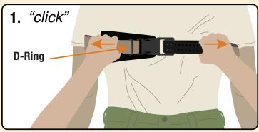
Apply the SJT to the patient under the arms, as high as possible. Place the D-ring on the injured side, aligning it with the side of the neck. Connect the buckle and secure the strap in place by pulling the **BROWN HANDLES** apart until you hear it click.
