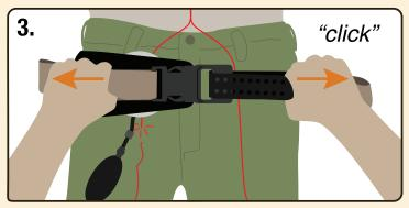
Pull the **BROWN HANDLES** away from each other until the buckle secures. You will hear an audible click. Fasten excess belt in place by pressing it down on the Velcro. You may hear a second click once the belt is secure.
